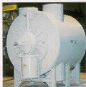
A 36-inch line size diverter for 25,000 gpm flow.
